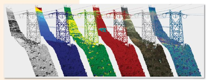
Fig. 3 Data visualized by (from left to right) reflectance, target range, multiple echoes ID, MTA confidence, true color, and pulse shape deviation
